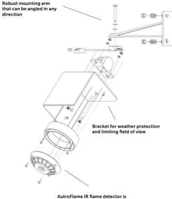
weather proof, has high false alarm immunity and provides accurate detection
