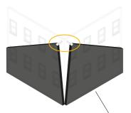
Recommended mounting: Horizontal mounting for optimal coverage of the facade.
