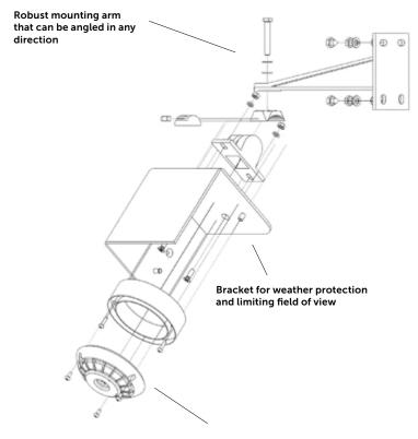
AutroFlame IR flame detector is weather proof, has high false alarm immunity and provides accurate detection
