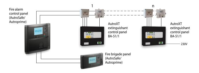
The AutroXT Extinguishant Control Panel BA-51/1 is connected to the AutroSafe 4 / Autroprime fire alarm control panel via two I/O units, each panel covering one zone.
